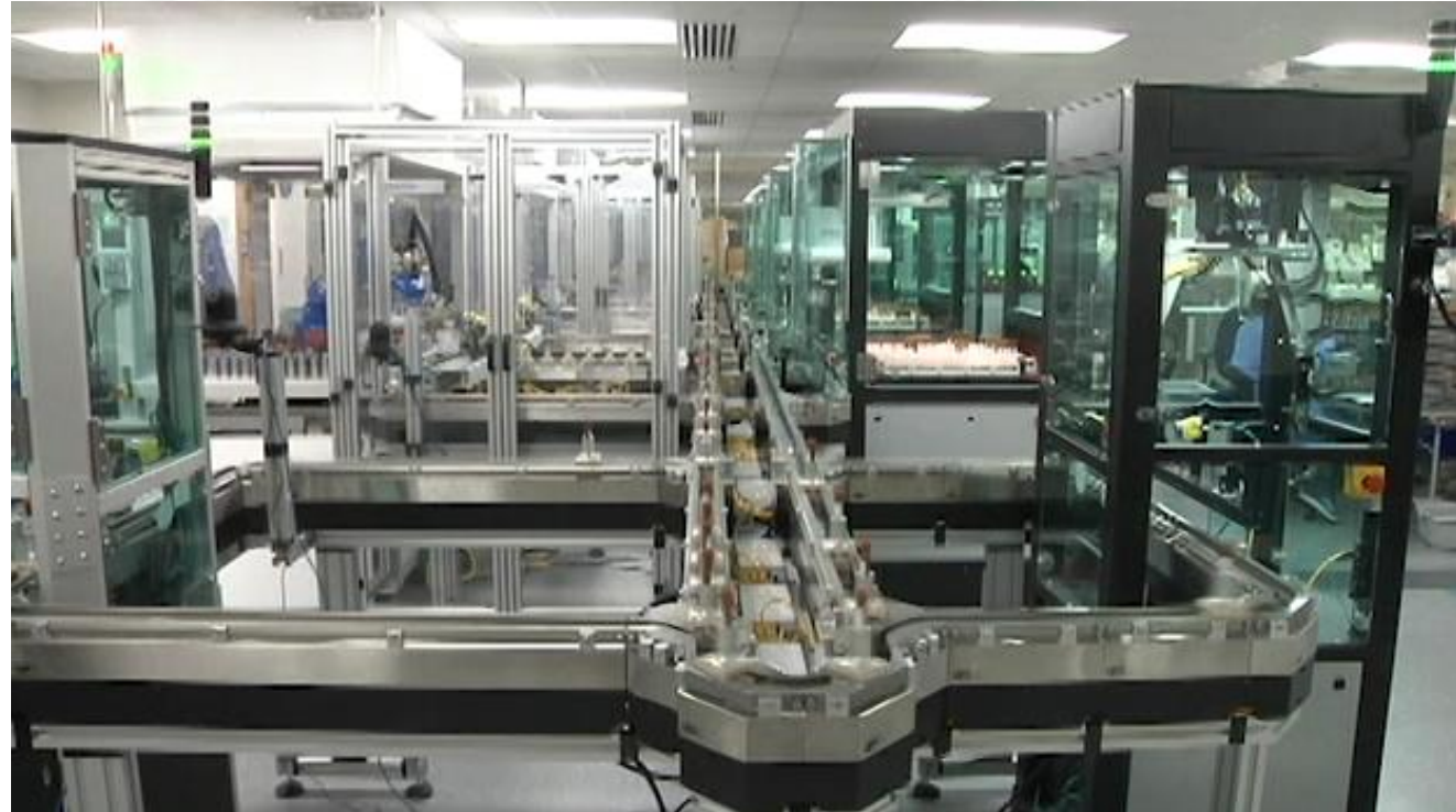
MagneMover LITE transporting vials of blood between testing stations
