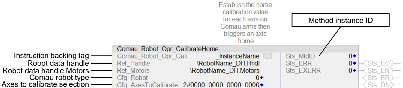
Most Comau robot servo axes are equipped with single turn, absolute encoders. The exception are the Comau Rebel SCARA robots. These are equipped with multi-turn, battery backed, absolute encoders. With the Rebels, Joint 1, 2, and 6 come from the factory calibrated. Joint 3 (the quill) would typically be the only axis that would need calibration using this instruction.
