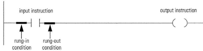
If the rung-in condition to an input instruction is true, the controller evaluates the instruction and sets the rung-out condition based on the results of the instruction. If the instruction evaluates to true, the rung-out condition is true; if the instruction evaluates to false, the rung-out condition is false.
