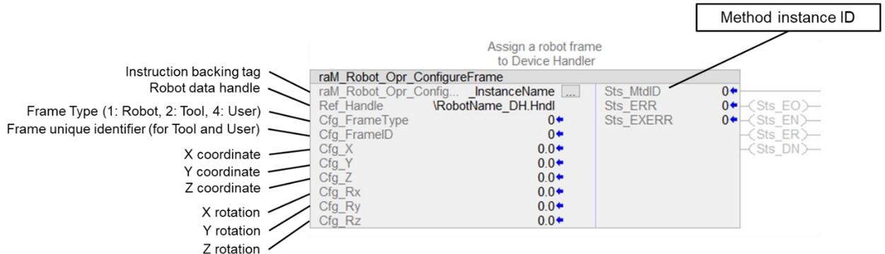
The Robot Device Handler has the capability by default to add 1 Robot frame, up to 15 User frames, and up to 15 Tool frames. It is not required to use all frames but a frame must be configured before it can be used in a move or zone instruction. Inputs X, Y, Z represent Cartesian offsets whereas input Rx, Ry, and Rz represent angular offsets in degrees and are solved in
